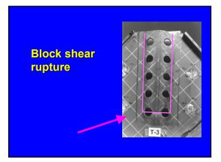
Failure (ult. load) is by tensile fracture at location shown, regardless of geometric proportions.
