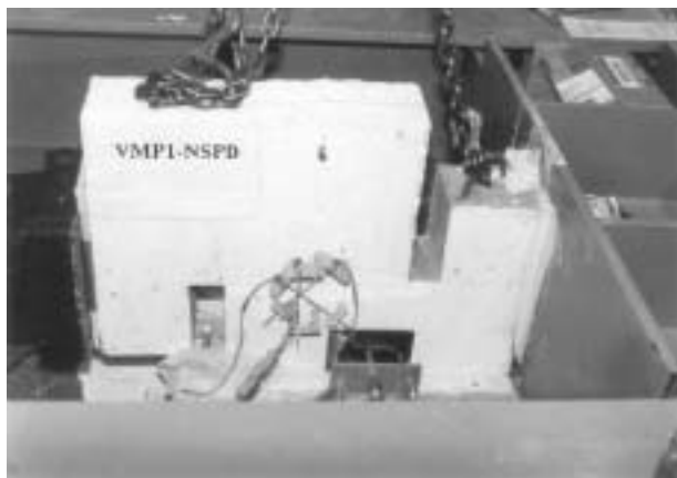
Fig. 4—Test setup of push-off specimens.
