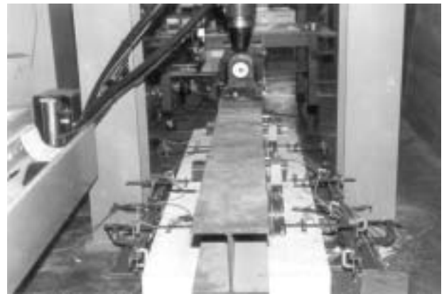
Fig. 15—Overall view of test setup and instrumented slab specimen.
