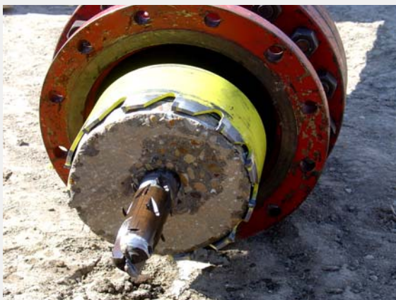
The coupon was studied to determine the needs for the larger 60-inch tap so that it would seat correctly.
