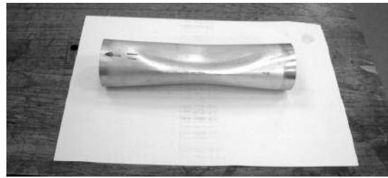
Figure 13: Ovaling of cylinder.
