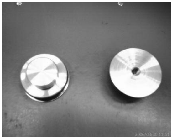
Figure 6: The end bungs or closure discs.
