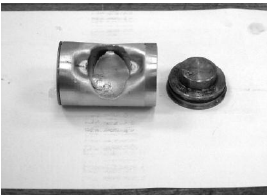
Figure 11: A closure disc with a buckled specimen.
