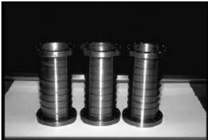
Figure 2: Ring-stiffened circular cylinders.
