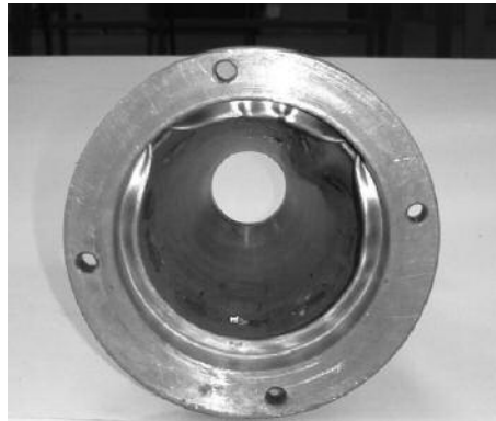
Figure 4: Axisymmetric collapse.
