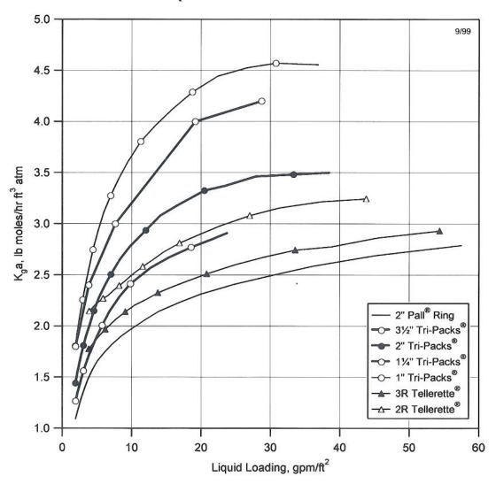
Tellerettes® data from Ceilcote Technical Bulletin 12-10.60. Column diameters and packed depths varied among the tests reported here.
