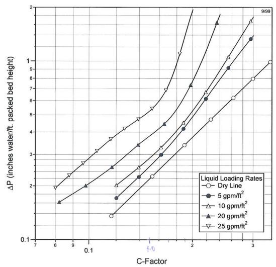
C-Factor =  $V_s[(\rho_V)/(\rho_L - \rho_V)]^{1/2}$  where V<sub>s</sub> = Superficial Vapor Velocity in ft/sec  $\rho_L$  and  $\rho_V$  = Density of Liquid and Vapor in lb/ft<sup>3</sup>
