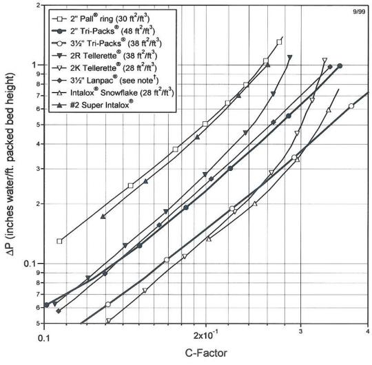
C-Factor =  $V_s[(\rho_V)/(\rho_L - \rho_V)]^{1/2}$  where  $V_s$  = Superficial Vapor Velocity in ft/sec  $\rho_I$  and  $\rho_V$  = Density of Liquid and Vapor in lb/ft<sup>3</sup>
