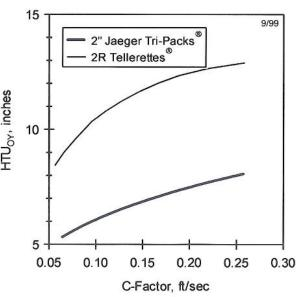
Tellerettes® HTU data from Ceilcote catalog 12-10.60; ∆p data from 12-10.11 Tri-Packs® HTU curves are simulations based on available HTU data from other systems.
