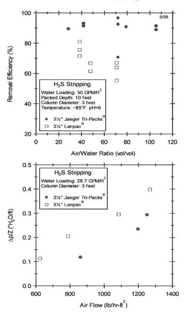
When Manatee County, Florida required H<sub>2</sub>S stripping towers for water treatment in 1992, they were concerned about long-term energy cost. The OEM Manufacturer retained by the county conducted tests on different packings to assure that their client received the most efficient packing and system. The partial results shown in the two graphs at the left show why they picked 3 1/2" Jaeger Tri-Packs® over 3 1/2" Lanpac® as the most efficient and affordable packing available.
