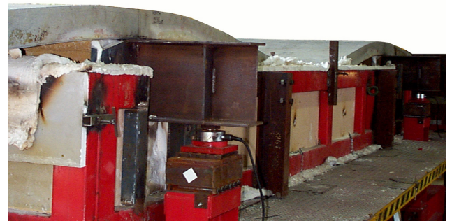
Fig. 3 Grossly-deformed continuous reinforced-concrete slab incorporating Class L mesh, after sustaining 2-hour Standard Fire Test without exhibiting steel fracture, while developing plastic hinges in critical moment regions
