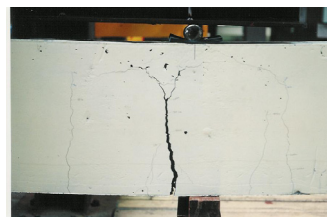
(b) Negative moment hinge (c) Positive moment hinge
