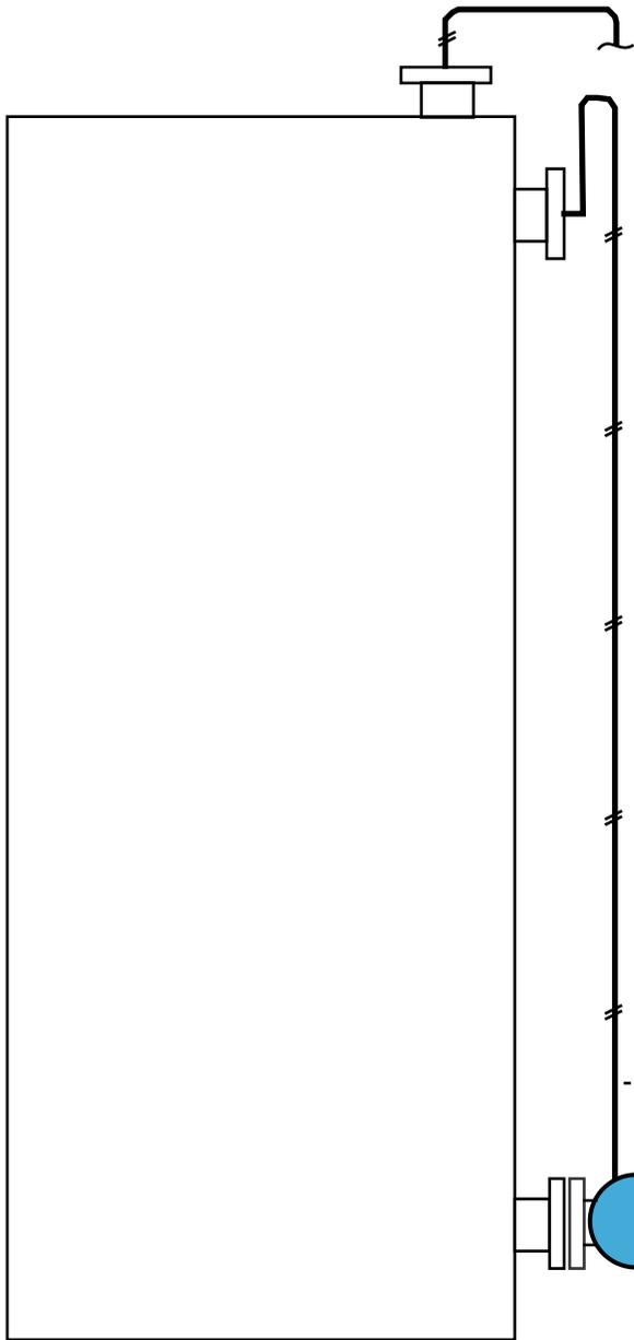
If you extend the LP tubing above upper tap by about 2 ft it prevents liquid entering on accidental overflow
