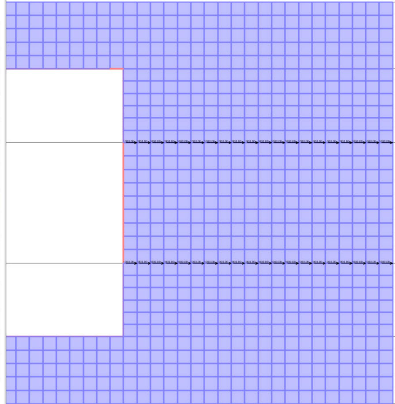
Loads applied along the web of the beam (where the weld between plate and beam occurs)
