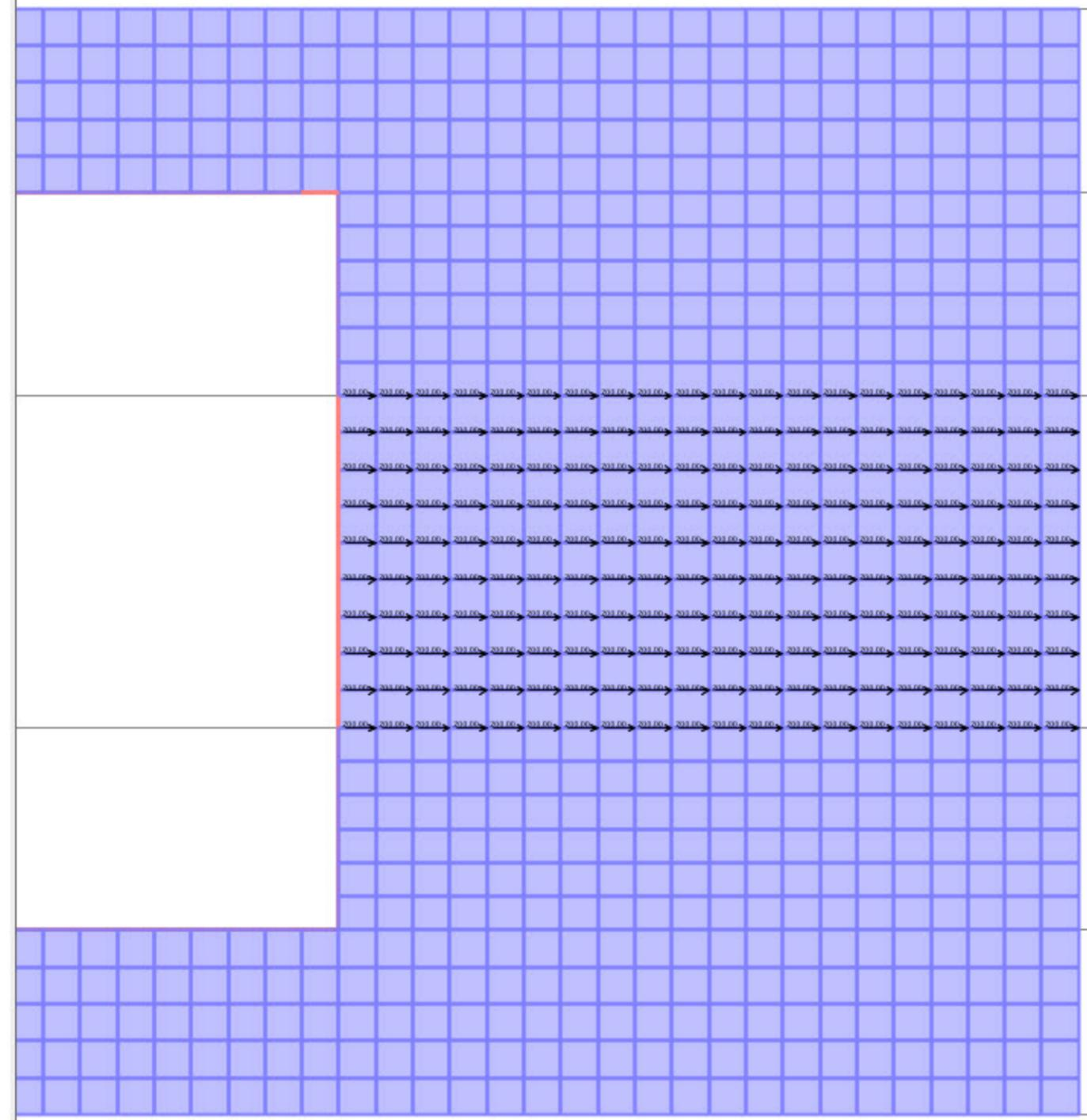
Loads applied all over where the plate is in contact with the beam.
