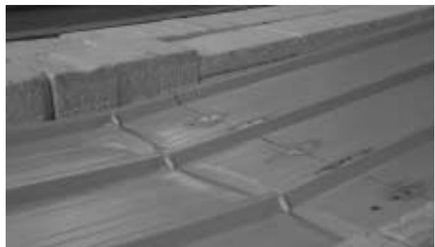
Figure 11 Typical Failure Mode of Tested Sandwich Panel
