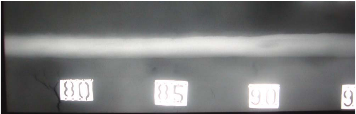
Figure 5 Porosity/pitting.
