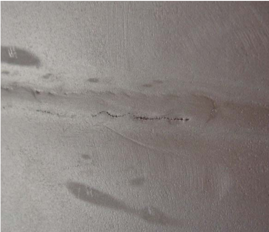
Figure 2– Porosity in weld seam
