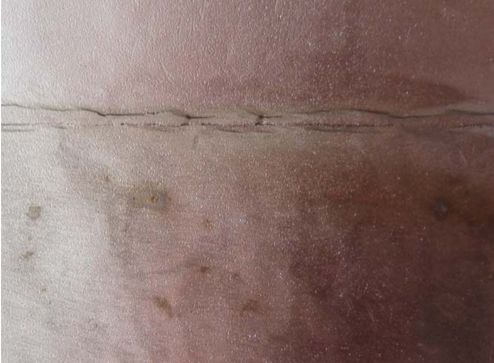
Figure 3 Undercut, LOP etc.
