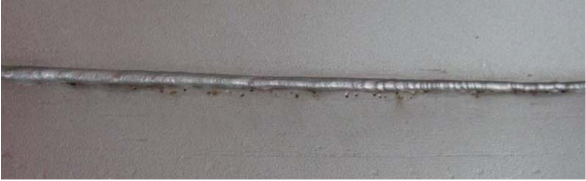
Figure 5 Porosity/pitting.
