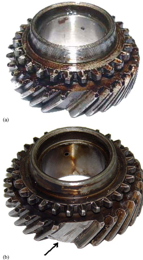
Fig. 5. (a) One tooth broken in the 2nd gear (defect-1), (b) Two teeth broken in 2nd gear (defect-2).
