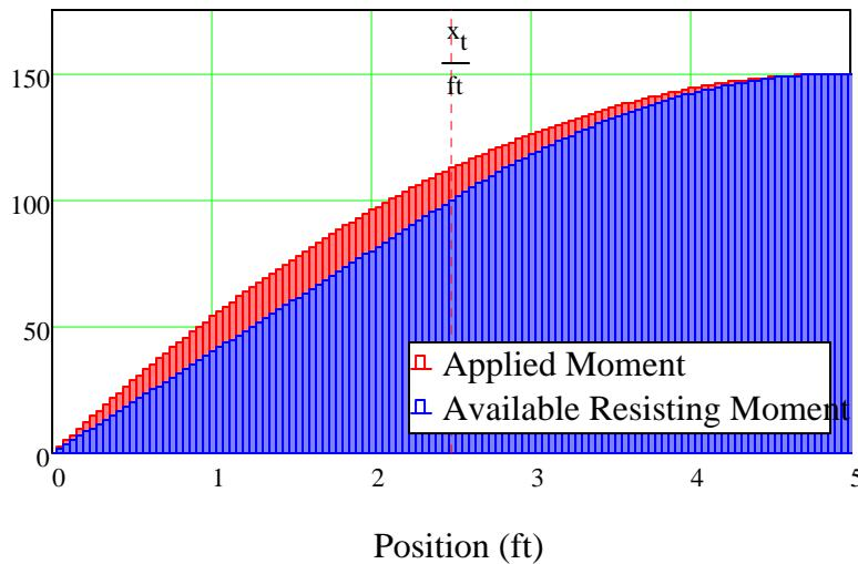
$w = 12 \frac{\text{kip}}{\text{ft}}$  Uniform load (develop plastic capacity at midspan).
