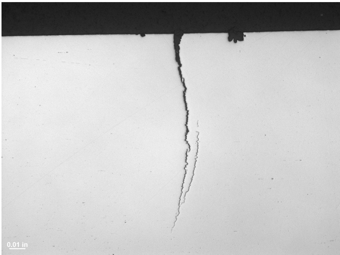
Photo 8. Overview of "spider crack" area, 25x, longitudinal section, as-polished
