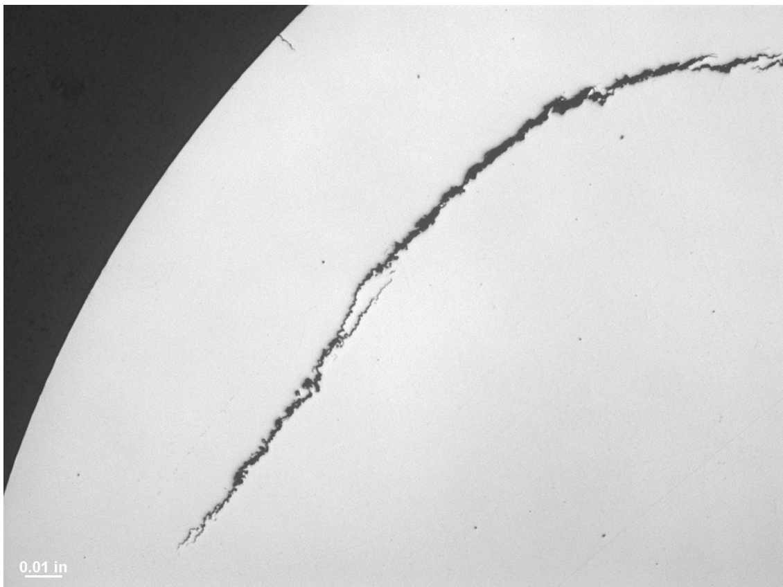
Photo 2. Continuation of photo 1 illustrating internal crack, 25x, transverse section, as-polished
