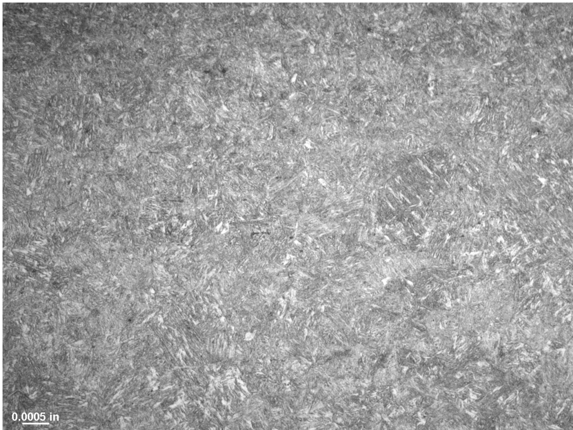
Photo 11. Typical appearance of core microstructure, 500x, transverse section, 2% nital etch.
