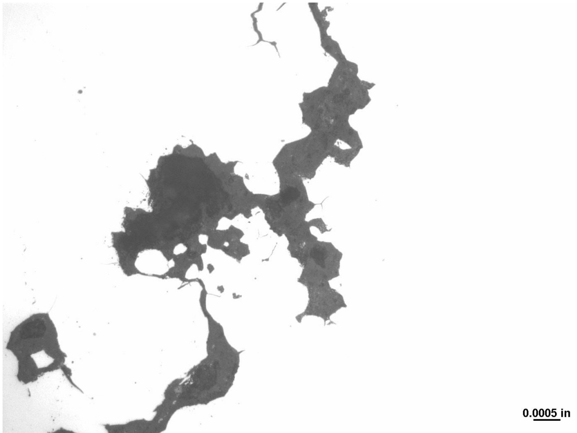
Photo 5. Closer view illustrating oxide inside the internal crack, 500x, transverse section, as-polished
