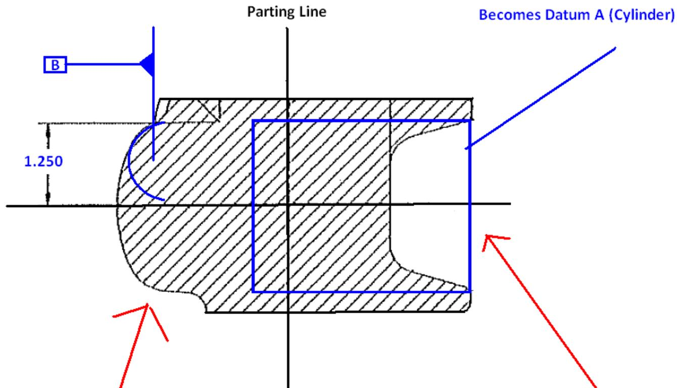
This side of parting line, value of Datum B to center line is within .005 (good)
