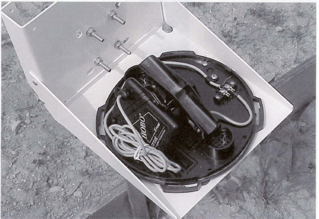
Figure A-4 Close-up View of Electronic Rain Gauge without cover
