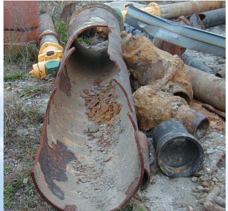
Corrosion continues until the pipe fails
