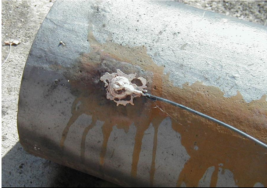
Exothermic Weld to Pit Cast Iron
