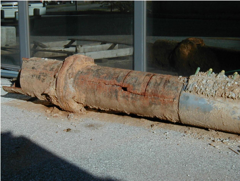
Graphitization weakens the cast iron pipe wall
