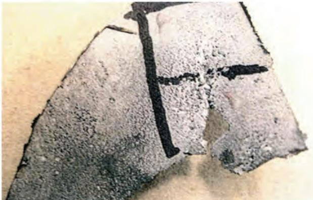
Figure 38. Aspect of Blade Surface under Direct Attack of Vortex Cavitation from Suction Recirculation. Cavitation Damage on the Pressure Side as a Large Crater Surrounded by Irregular Pitting.
