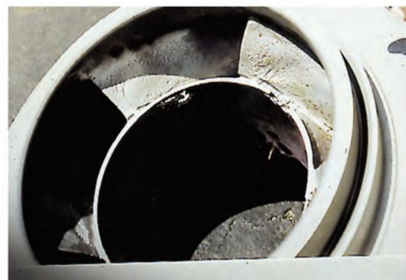
Figure 41. Cavitation Damage Combined from Sheet Cavitation (Suction Side) and Corner Cavitation.
