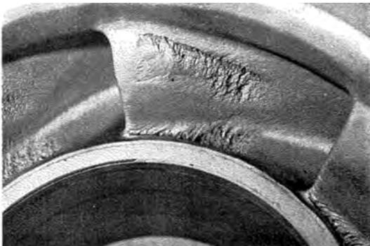
Figure 35. Cavitation Damage on Suction Side (Front or Visible) of Impeller Blade. (Courtesy of Cooper and Antunes, 1982)
