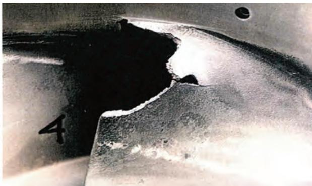
Figure 39. Blade Breakage Caused by Vortex Cavitation from Suction Recirculation (Operating Time: 525 Hours, Impeller Material: CF3M). Hole with Net Contour Produced from Vortex Acting on Backside.
