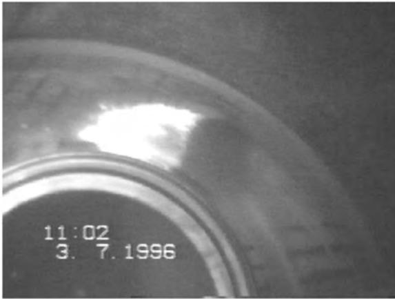
Figure 1. Sheet Cavity on Centrifugal Pump Impeller Vane Leading Edge. (Courtesy of Visser, et al., 1998, Turbomachinery Laboratory)
