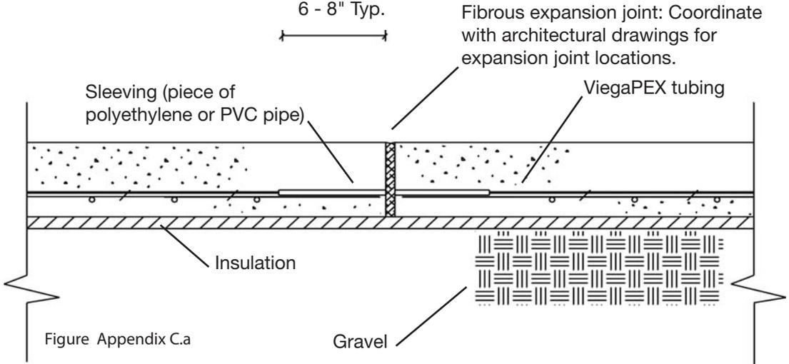
**SECTION THRU METAL EXPANSION JOINT (TYPICAL)**
