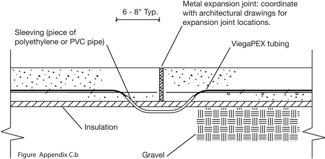
**SECTION THRU CONTROL JOINT (TYPICAL)**
