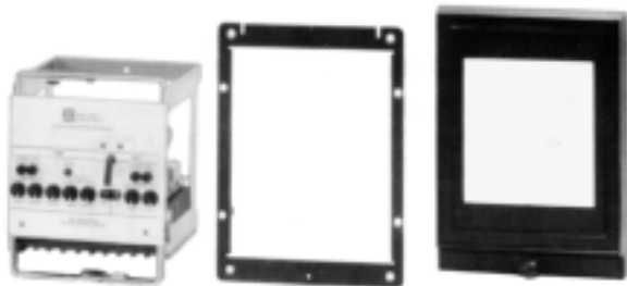
The BE1-50/51B-214 retrofit kit consists of a relay cradle, an adapter plate, and a cover. It allows plug-in installation in an existing IAC case without making any wiring changes.
