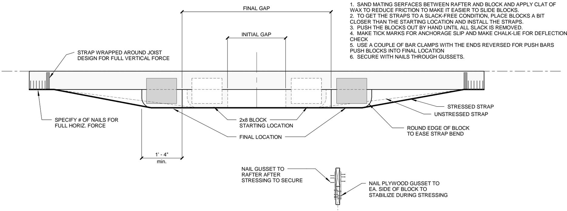
1. SAND MATING SURFACES BETWEEN RAFTER AND BLOCK AND APPLY CLAY OF WAX TO REDUCE FRICTION TO MAKE IT EASIER TO SLIDE BLOCKS.
