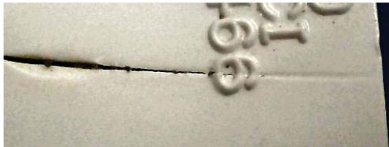
Figure 6: Stretch mark at end of a crack.
