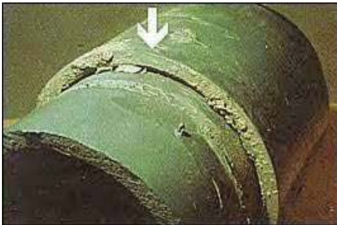
Figure 22: Insufficient Solvent cement was used.
