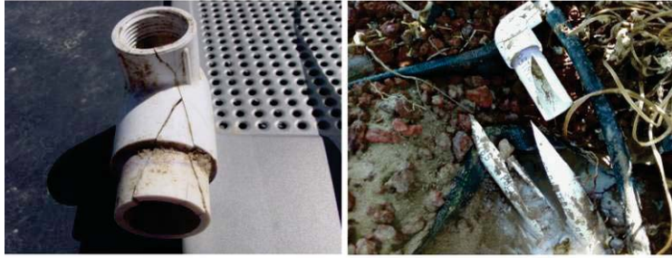
Figure 7: Breaks due to freezing water
