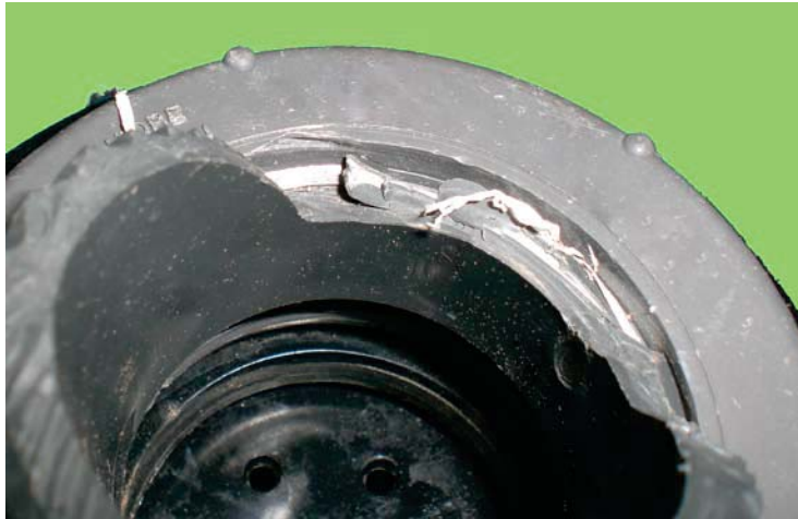
Figure 9: Vibration failure of male threads.
