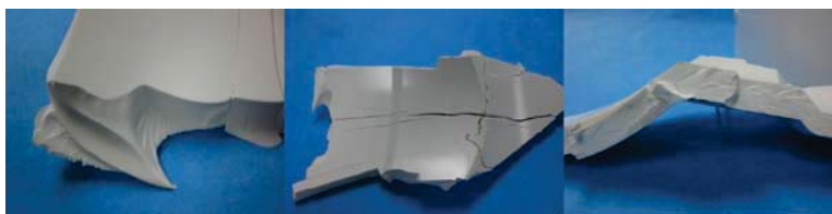
Figure 1: Typical burst or short term failure
