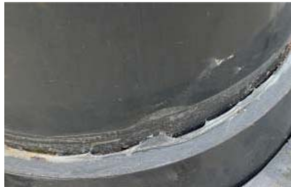
Figure 12: Assembly was moved during cure time.
