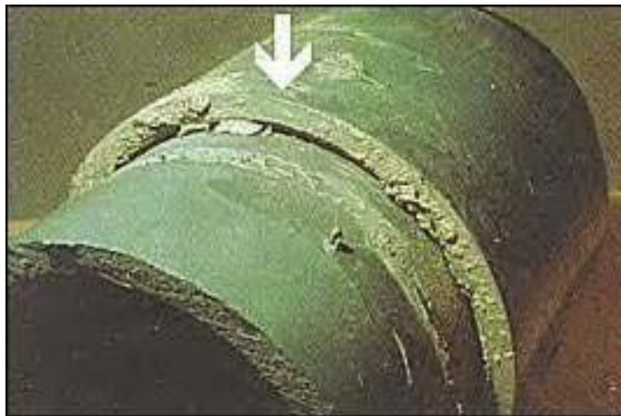
Figure 22: Insufficient Solvent cement was used.
