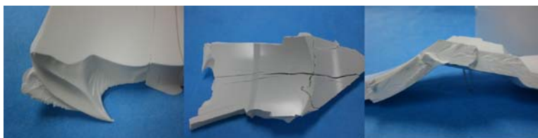
Figure 1: Typical burst or short term failure
