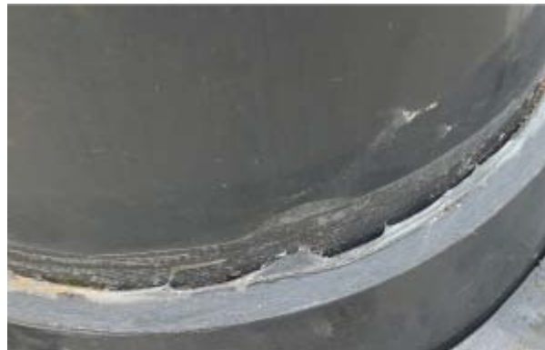
Figure 12: Assembly was moved during cure time.
