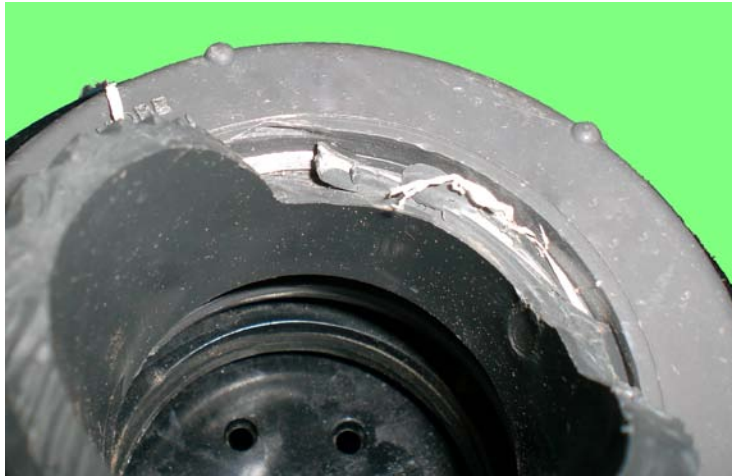
Figure 9: Vibration failure of male threads.
