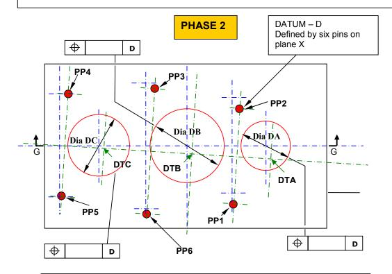
Green lines- Best fit of marker K to the centers of pins PP1 to PP6 (Marker K when applied best fit had a translation and rotation). Check the distances between the centers of circles-holes (each one)
