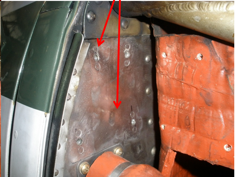
Deformation surrounding upper R/H engine frame attachment to firewall.
