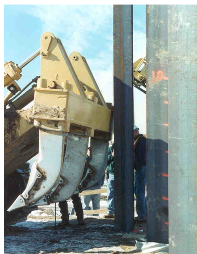
Figure 7. Applying lateral load to pile.
