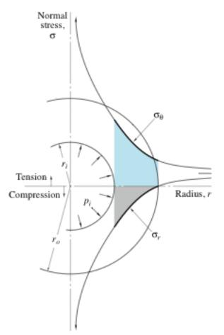
Internally pressurized, thick-walled cylinder showing circumferential (hoop) and radial stresses for various radii (Hamrock, Schmid, & Jacobson - <u>Fundamentals of Machine Design</u>)
