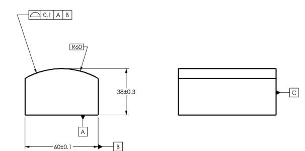
Since no basic diameter dimension is included, does the profile tolerance impose a tolerance zone that is the same as cylindricity?
