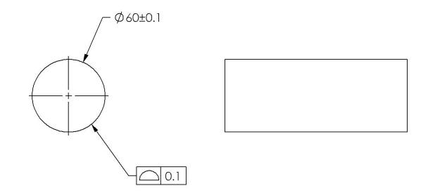
Now with a pin that has an elliptical cross-section, how does this work?
