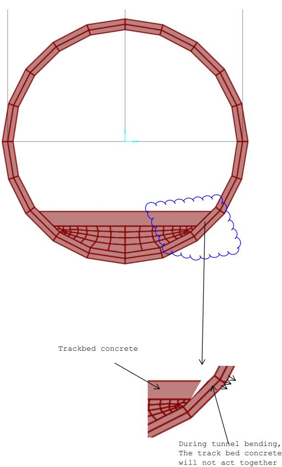
The track bed concrete will not act together with tunnel after attaining some tension limit.hence there will be a gap as shown how model this in spring?
