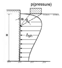
$\alpha$  = angle between foundation wall and a line connecting the point on the wall under consideration and a point on the bottom corner of the footing nearest to the wall (rad.)
