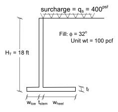
Natural Soil: φ = 32° allowable bearing pressure = 5000psf
