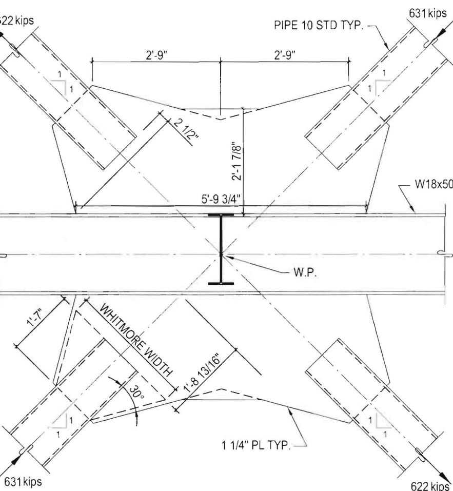
**Design the weld at the gusset/beam interface**
