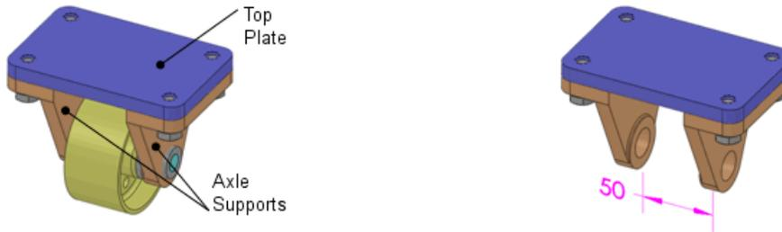
The assembly includes axle supports that are fastened to the top plate using 10 mm bolts. The measurement to evaluate is the minimum and maximum distance between the inner faces of the axle supports.
