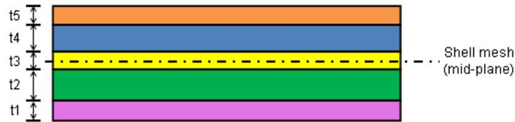
You can use composite materials for linear static, frequency, and buckling studies. The plies are assumed to be perfectly bonded with no bonding thickness and negligible shear deformation between them.
