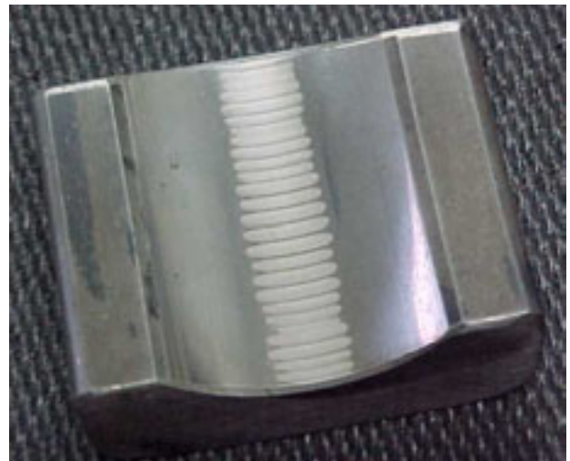
Figure A2-2: Fluting on a ball bearing outer race.
