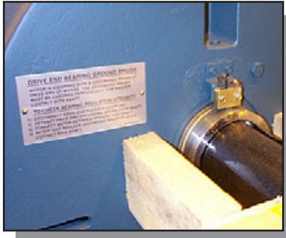
Figure 26: Shaft grounding brush.
