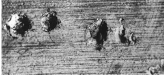
Figure 12: Fusion craters in a bearing race from Scanning Electron Microscope image.
