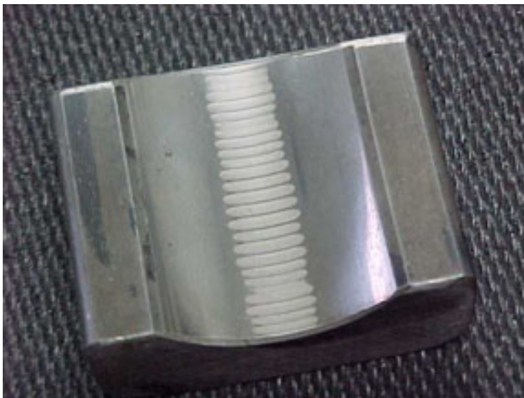
Figure 13: Bearing race fluting.
