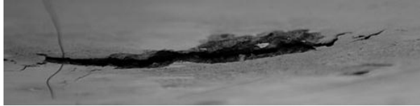
Fig. 4.2: Punching damage at the bottom of a slab after an experiment.
