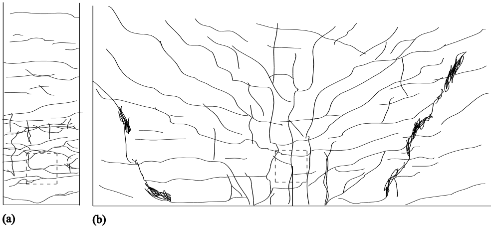
Fig. 4.1: Difference in cracking pattern between a beam and a slab: (a) cracking pattern at bottom face after BS2T1, (b) cracking pattern at bottom face after S9T1. The dashed lines denote the location of the loading plate. Bolder lines in (b) denote areas of punching damage. Note that the cracks further than the inner face of the support are not drawn in this sketch.
