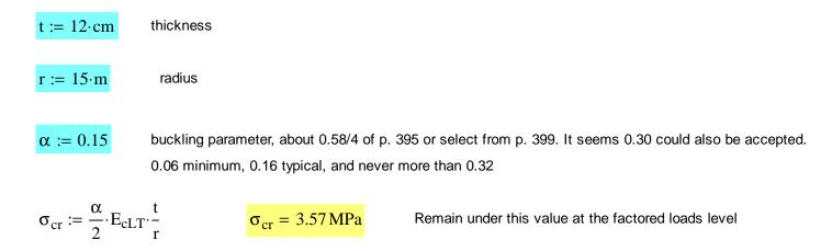
Note this formulation of the buckling risk seems not consistent with that of cylindrical shells, which portrait as unsecure when compared to spherical domes, even the differences of loading (radial pressure on the shell for the dome and longitudinal compression for the cylinder) are accounted for.
