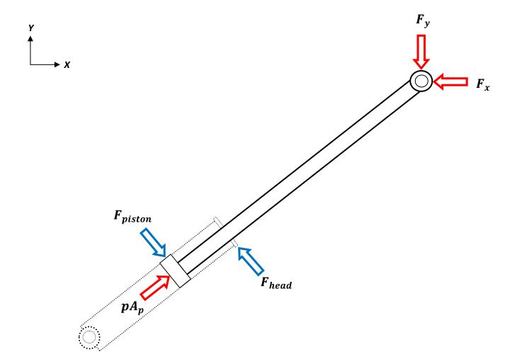
I want to evaluate the sideload on the rod. Therefore I need to calcultate  $F_{head}$ .
