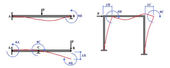
In 2 dimensions, such as the figures shown, each node can have a maximum of 2 displacements and 1 rotation ( $\Delta x$ ,  $\Delta y$  and  $\theta$ ). For the frame above; if  $\Delta B = \Delta C$ , then these would only cont s 1 unknown.
