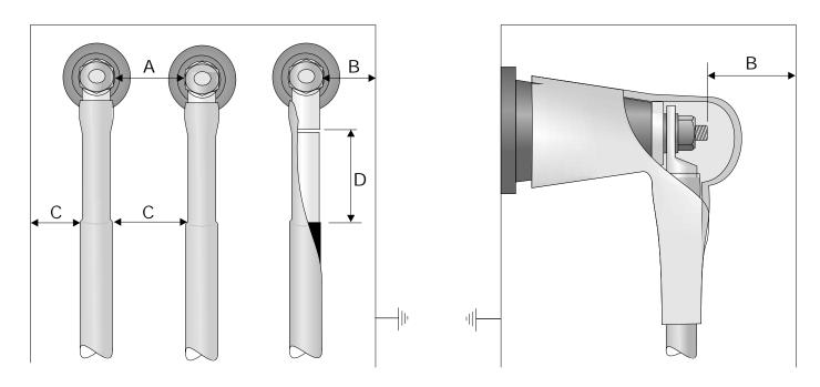
Check the cable box for minimum clearances and refer to table 1 below. If actual dimension 'A' and 'B' is less than the value given, a bushing boot must be fitted.
