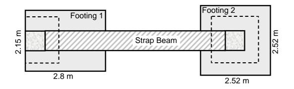
Estimate d' for footing 1 by 3-way punching shear under column 1 Using <u>Structural Depth of Concrete</u> table for punching shear failure, with  $P_{u1} = 890 \text{ kN}, f_c' = 24 \text{ MPa} \text{ and } p' = 2/ + w = 2(0.4) + 0.4 = 1.2 \text{ m}, \text{ the}$ value of **d'**  $\approx$  **0.35 m**
