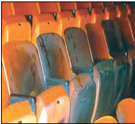
Figure 3: Heat damage of seats at level above fire.
