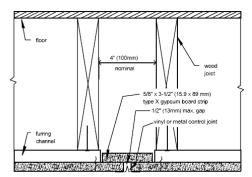
CONTROL JOINT PARALLEL TO FRAMING WITH FURRED CEILING
