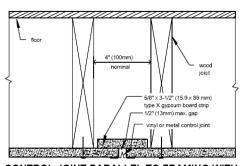
CONTROL JOINT PARALLEL TO FRAMING WITH DIRECT-ATTACHED CEILING
