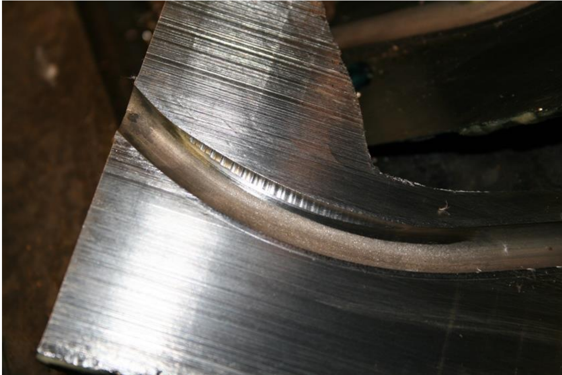
Camera 7551 showing wear in the S-Tube
