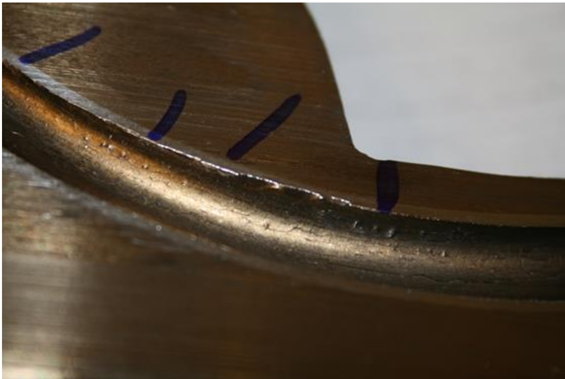
Camera C1137-D09 showing cracks and interior wall defects in the S-Tube
