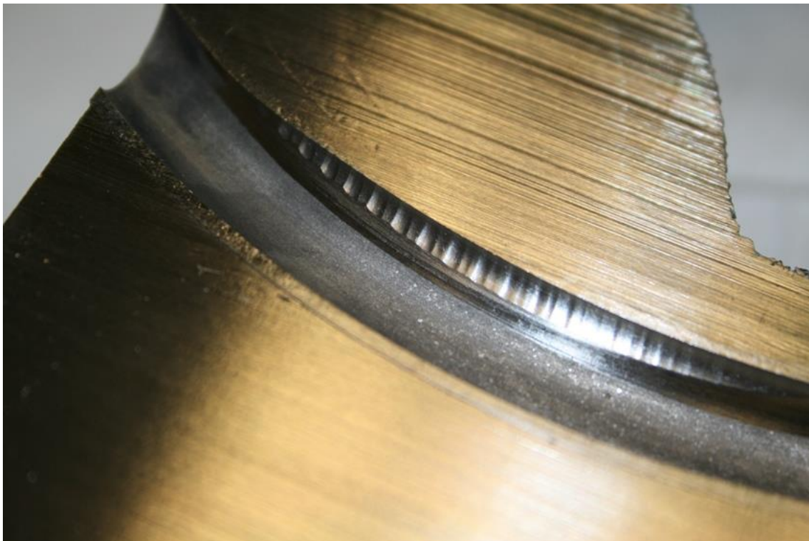
Camera 7551 showing wear in the S-Tube
