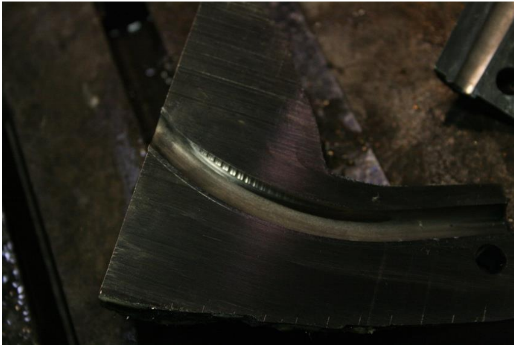
Camera 7551 showing wear in the S-Tube
