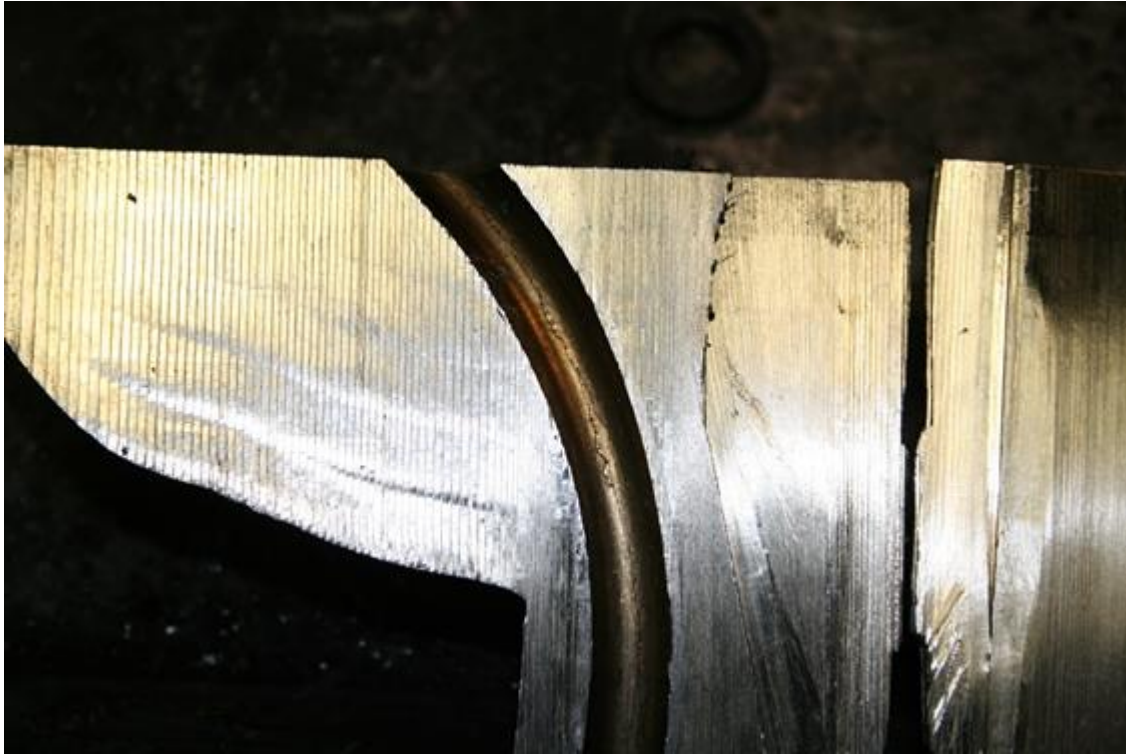
Camera C1137-D09 showing cracks in the S-Tube
