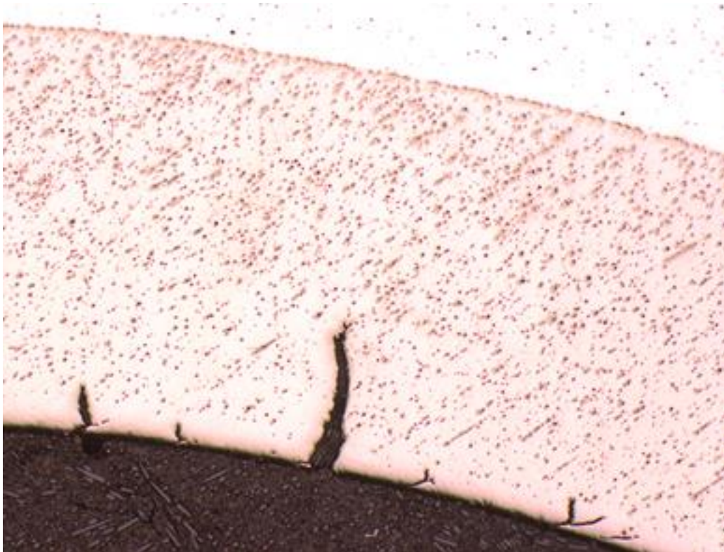
Micrograph of Camera C1137-D09 showing cracks on the interior wall of the S-Tube
