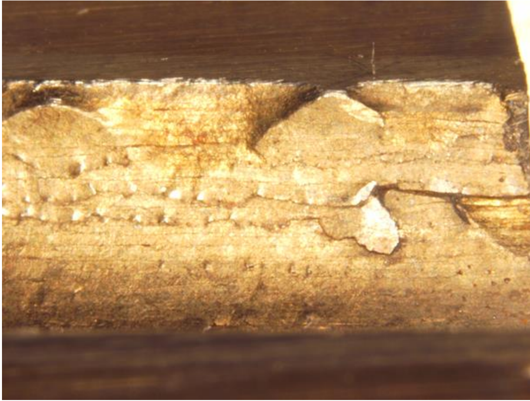
Higher magnification of Camera C1137-D09 showing cracks and interior wall defects in the S-Tube
