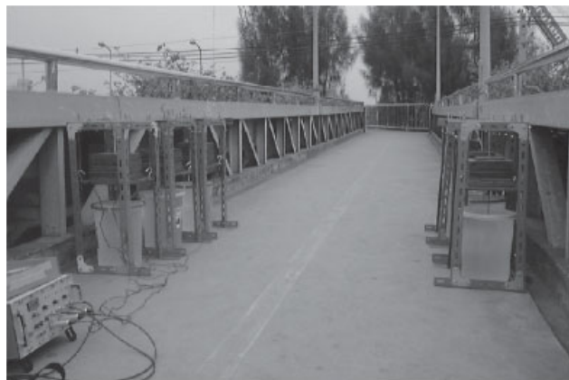
Figure 10. Non-linear MTMDs on a pedestrian bridge.
