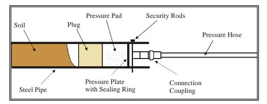
Figure 4-7: Spoil removal with compressed air (Mole Engineering, UK)
