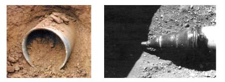
Figure 4-4: Left: Open-end pipe (TT Technologies). Right: Closed-end pipe on an 8-in pipe using multiple reducers (Vermeer)
