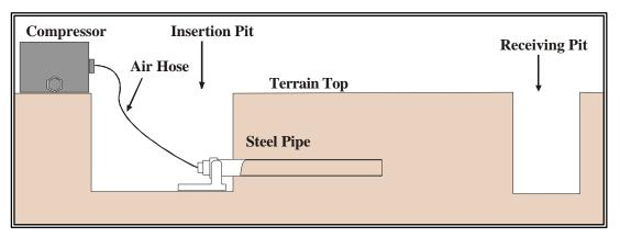
Figure 1-1: Typical pipe ramming setup
