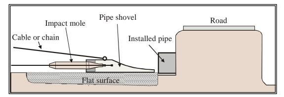
Figure 4-9: Spoil removal using a fabricated pipe shovel (Vermeer)
