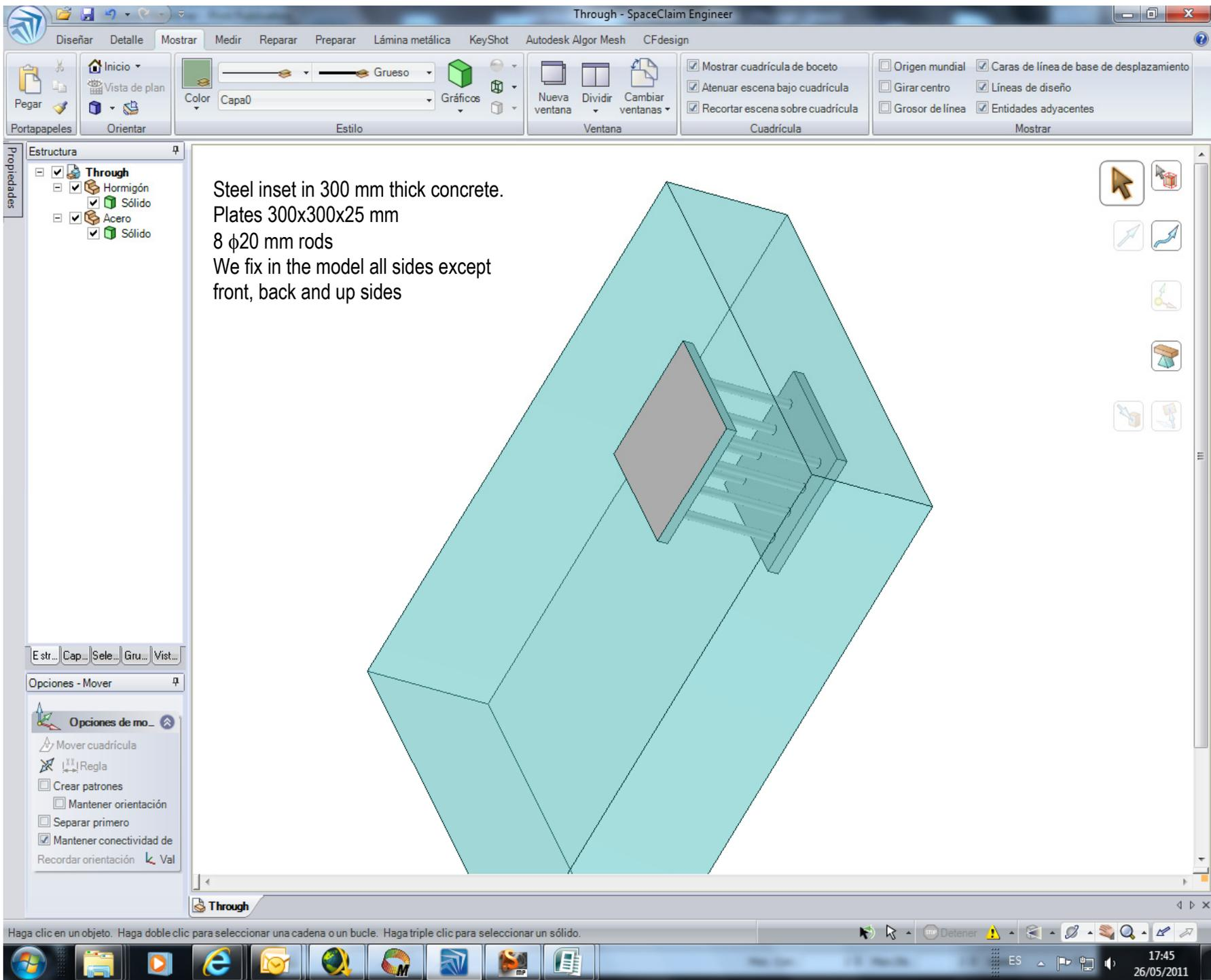
Steel inset in 300 mm thick concrete.
