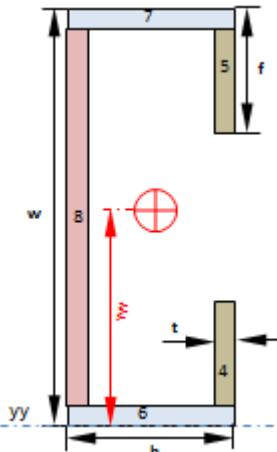
$$I_4 := \frac{(d_1 \cdot b_1^3)}{12} = (9.374 \cdot 10^{-8}) \text{ m}^4 \quad d_{y4} := d_{c4} - y_{yy} = -0.079 \text{ m}$$
