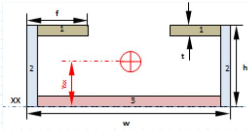
$$b_1 := (f - t) = 0.052 \text{ m} \quad d_1 := t = 0.008 \text{ m}$$
