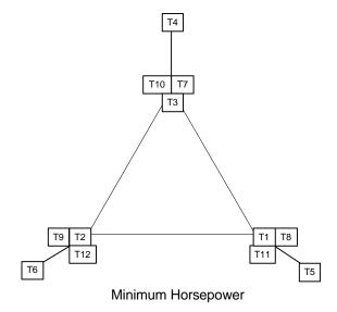
To reverse direction of rotation interchange connections L1 and L2.
