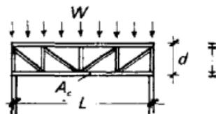
$\frac{M}{dA_c} < p_c$  where  $M$  is working value of bending moment on truss at midspan
