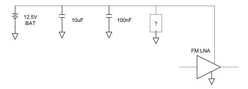
This amplifier is powered with the battery of the car. Doesn't have regulation.
