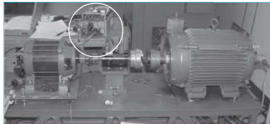
Figure 1. Regenerative drive and load motor dynamometer test setup. The AC vector drive is circled.
